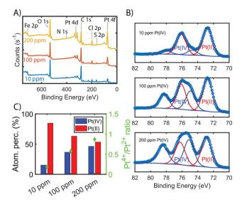
Fig. 4 (A) shows the wide XPS scan with elemental labelling of Fe-BTC/PDA-DIP-7.3 soaked in Pt(IV) solutions with increasing concentration (10, 100, 200 ppm, 1 mg ml<sup>-1</sup>, 6 hours adsorption time). (B) Fitted Pt 4f XPS data for Fe-BTC/PDA-DIP-7.3 soaked in Pt(IV) solutions with increasing Pt concentration. (C) The relative percentage of adsorbed Pt(IV) and Pt(II) are calculated from the synthetic peak areas of the fitted Pt(IV) and Pt(II)  $4f_{7/2}$  and  $4f_{5/2}$  doublets in (A).
