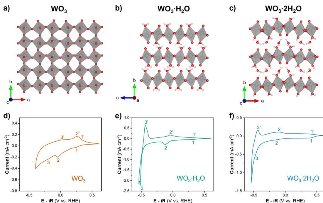
Fig. 2 Crystal structures of (a) monoclinic  $\text{WO}_3$ , (b) orthorhombic  $\text{WO}_3 \cdot \text{H}_2\text{O}$ , and (c) monoclinic  $\text{WO}_3 \cdot 2\text{H}_2\text{O}$ .<sup>51</sup> Cyclic voltammograms of (d)  $\text{WO}_3$ , (e)  $\text{WO}_3 \cdot \text{H}_2\text{O}$ , and (f)  $\text{WO}_3 \cdot 2\text{H}_2\text{O}$  with a rotation rate of 1600 rpm and scan rate of  $10 \text{ mV s}^{-1}$  in  $0.5 \text{ M H}_2\text{SO}_4$ .
