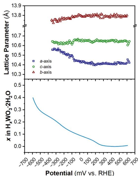
Fig. 11 Trend of lattice parameters (from Pawley refinements of the operando XRD) and proton composition in  $\text{H}_x\text{WO}_3 \cdot 2\text{H}_2\text{O}$  (from Fig. 5e) as a function of potential during the cathodic cyclic voltammetry scan in  $0.5 \text{ M H}_2\text{SO}_4$  at  $10 \text{ mV s}^{-1}$ .
