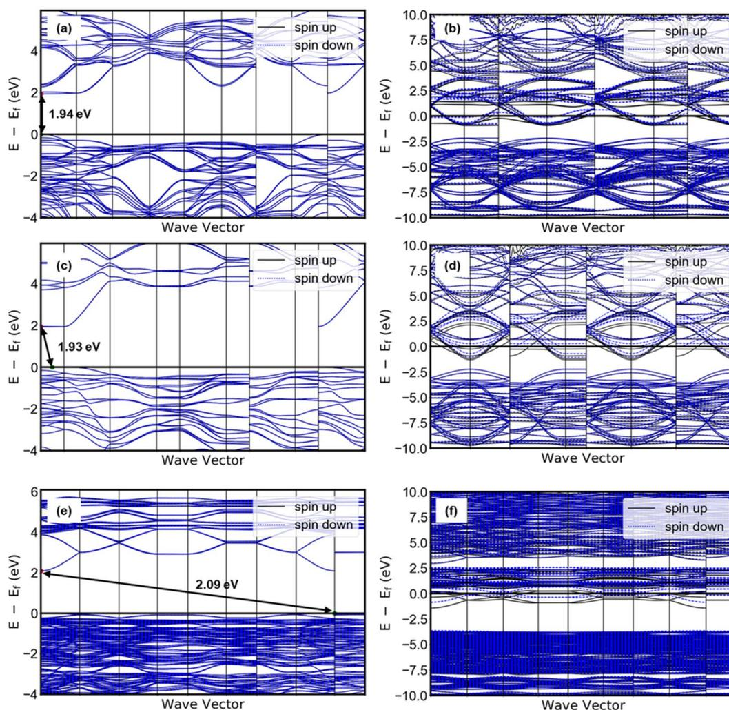
Fig. 12 Band structure of pristine (left) and protonated (right) tungsten oxides: (a)  $\text{WO}_3$ , (b)  $\text{H}_{0.5}\text{WO}_3$ , (c)  $\text{WO}_3 \cdot \text{H}_2\text{O}$ , (d)  $\text{H}_{0.5}\text{WO}_3 \cdot \text{H}_2\text{O}$ , (e)  $\text{WO}_3 \cdot 2\text{H}_2\text{O}$ , (f)  $\text{H}_{0.5}\text{WO}_3 \cdot 2\text{H}_2\text{O}$ .
