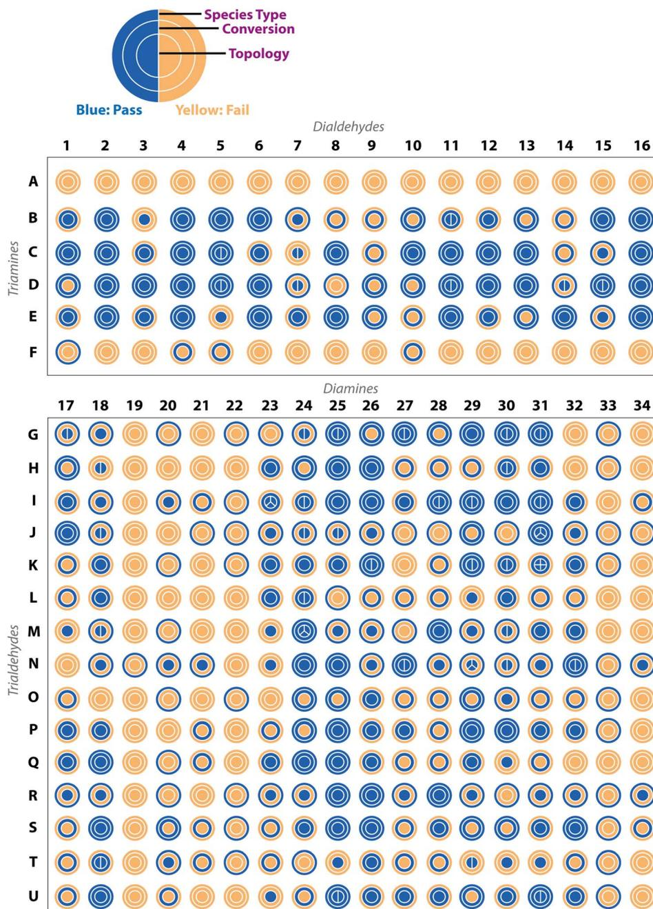
Fig. 5 Experimental results for all 366 precursor combinations from the automated analysis, based on either 'pass' (blue) or 'fail' (yellow) of the computer vision turbidity analysis,  $^1\text{H}$  NMR spectroscopy, and high-resolution mass spectrometry (HRMS), to indicate the species type, conversion, and cage topology, respectively. The splitting of the inner ring indicates the number of cage topologies identified by HRMS.
