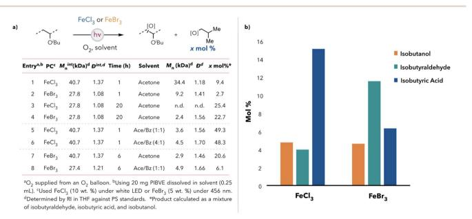
Fig. 1 (a) Table for the PIBVE degradation results for FeCl<sub>3</sub> and FeBr<sub>3</sub>. (b) Small molecule distributions for FeCl<sub>3</sub> and FeBr<sub>3</sub> catalyzed degradation in acetone after 20 h.
