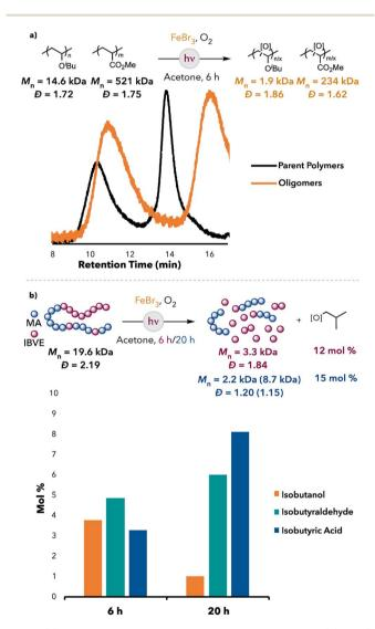
Fig. 5 (a) PIBVE and PMA mixture degradation with FeBr<sub>3</sub>. (b) Poly(-IBVE-co-MA) degradation results: Lower  $M_n$  peak (higher  $M_n$  peak).
