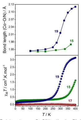
Fig. 4 (Top) change in average Co-O/N bond length vs. T for 15.BPh<sub>4</sub> (green squares) and 19.BPh<sub>4</sub> (blue squares); and (bottom) plot of  $\chi_M T$  vs. T for the first heating of 15.BPh<sub>4</sub> (green spheres), 19.BPh<sub>4</sub> (blue spheres) and 17.BPh<sub>4</sub> (red spheres).
