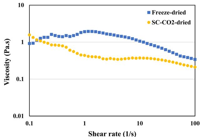
Fig. 7 Viscosity of freeze-dried and SC-CO<sub>2</sub>-dried sorghum proteins at 20 °C with a pH of 12.
