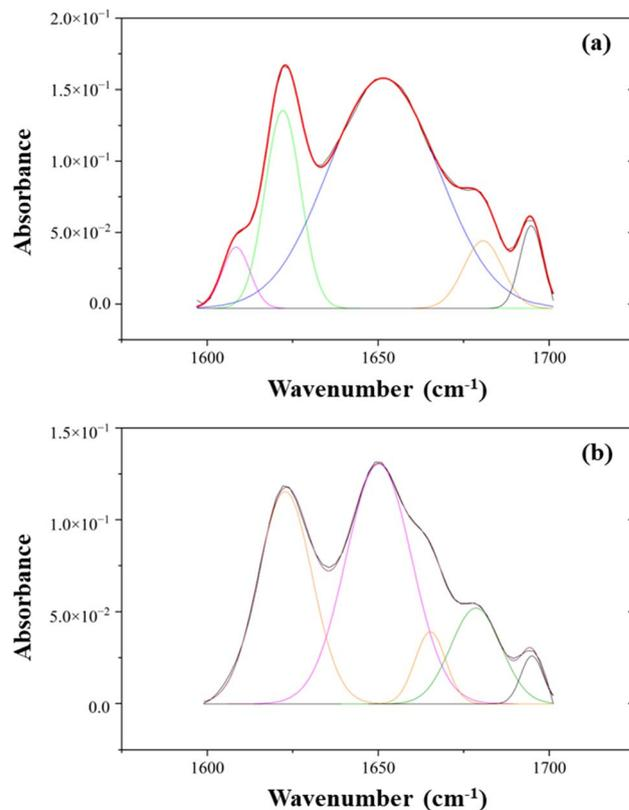
Fig. 6 The peak-fitted ATR-FTIR spectra of (a) freeze-dried and (b) SC-CO<sub>2</sub>-dried sorghum proteins in the range of 1600–1700 cm<sup>-1</sup>.
