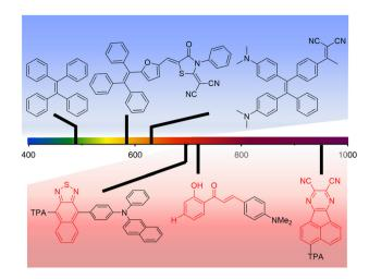
Fig. 5 Examples of chemical structures of AlEgens with emissive properties in different spectral regions (TPA = triphenylamine). Blue background: UV-vis responsive AlEgens proposed in the LSC literature (ref. 41, 43 and 45 from left to right); red background: chemical platforms to be potentially employed for DR/NIR-responsive LSCs (ref. 57-59 from left to right).
