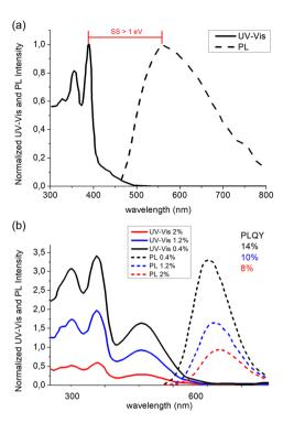
Fig. 3 (a) UV-Vis (solid) and PL (dashed) spectra in PMMA matrix of compound 2. (b) UV-Vis and PL spectra of compound 6 in PMMA matrix at concentrations of 0.4% (black), 1.2% (blue) and 2% (red) respectively. Partially reproduced from ref. 42 and 47. Copyright 2015 and 2022 Wiley.
