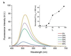
Fig. 4 (a) UV-vis spectra of dilute solutions of 16 in THF-H<sub>2</sub>O mixtures with different volume fractions of water ( $f_w$ ). (b) PL spectra of 16 in THF-H<sub>2</sub>O mixtures at different fw values. The inset shows the normalized PL intensity at as fw changes. Partially reproduced with permission from ref. 55. Copyright 2021 Wiley.
