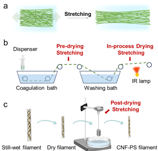
Fig. 9 Schematic presentation of (a) CNF network changes practically the CNF orientation during the wet stretching process, (b) pre-drying and in-process stretching processes and the (c) post-drying stretching process. 51 Adapted with permission from ref. 51. Copyright 2023 Elsevier.
