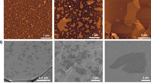
Fig. 1 Morphological characterization of us-GO, s-GO and I-GO. (A) Height atomic force microscopy (AFM) images. (B) Scanning electron microscopy (SEM) images.
