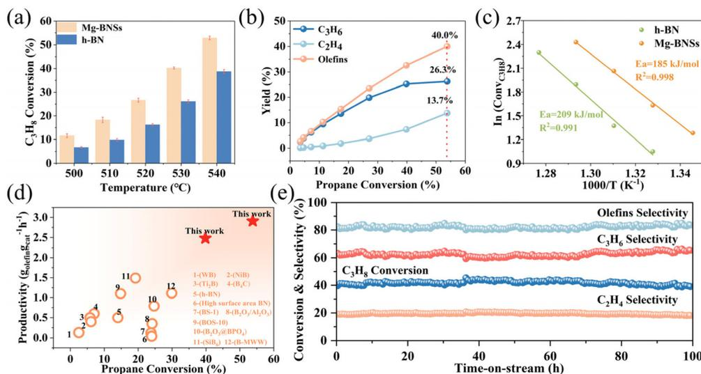
**Fig. 3** (a) Catalytic performance of Mg-BNSs and commercial h-BN at different temperatures. (b) Olefin yield as a function of propane conversion over Mg-BNSs. (c) Arrhenius plots of Mg-BNSs and commercial h-BN. (d) Comparison of Mg-BNSs with the reported boron-based catalysts. See Table S3† for specific values. (e) Stability test of Mg-BNSs at 530 °C. Reaction conditions: atmospheric pressure,  $C_3H_8/O_2/N_2$  ratio = 1 : 1 : 3, and WHSV = 24 000 ml  $g^{-1} h^{-1}$ .
