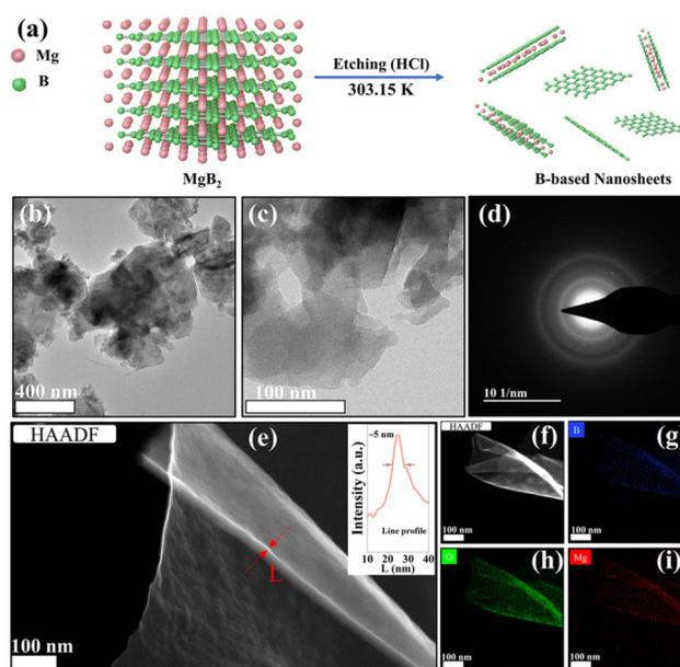
**Fig. 1** (a) Schematic illustration for the preparation of boron-based nanosheets. (b) TEM image of  $\text{MgB}_2$ . (c) TEM image of Mg-BNSs. (d) SAED pattern of Mg-BNSs. (e) HAADF of a thin nanosheet. The inset image is the line profile at position "L". (f–i) EDS mappings of a thin nanosheet.
