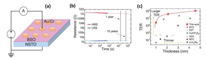
Fig. 7 (a) Schematic diagram of a 4.6-nm-thin ferroelectric  $Bi_{1.8}Sm_{0.2}O_3$  (BSO) FeTJ device structure and (b) retention measurement indicating prolonged retention for more than 10 years by extrapolation. (c) Comparison of tunnelling electroresistance (TER) values of the BSO FTJ device with other ferroelectric materials and thicknesses.<sup>34</sup>
