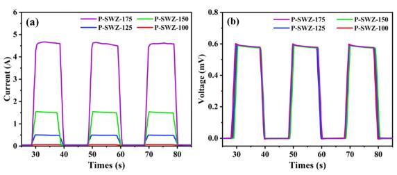
Fig. 9 The photodetector response of SWCNT/ZnO NCs: (a) current and (b) voltage.
