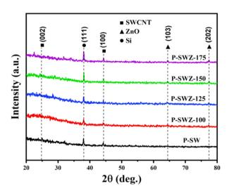
Fig. 2 Diffraction patterns of SWCNT and SWCNT/ZnO NC integrated Si thin film.
