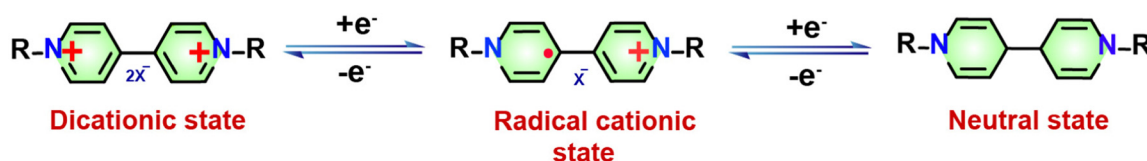
Scheme 1 Schematic representation of different redox states of a viologen moiety. The viologen moiety undergoes two reversible reduction reactions. The dicationic state of the viologen moiety is the most stable state of viologen. [R = alkyl/aromatic].
