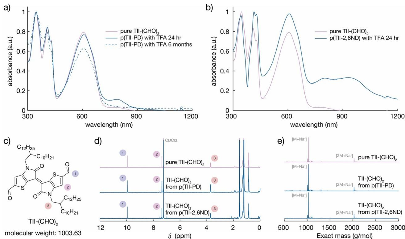
**Fig. 4** Comparison of the pure and recycled TII-(CHO)<sub>2</sub>: UV-vis-NIR absorption spectra of decomposed (a) p(TII-PD) and (b) p(TII-2,6ND) solutions after adding TFA solution, (c) the chemical structure and exact mass of TII-(CHO)<sub>2</sub>, (d) <sup>1</sup>H-NMR assignment of recycled TII-(CHO)<sub>2</sub> from p(TII-PD) and p(TII-2,6ND), and (e) ESI-HRMS spectra of recycled TII-(CHO)<sub>2</sub> from p(TII-PD) and p(TII-2,6ND).
