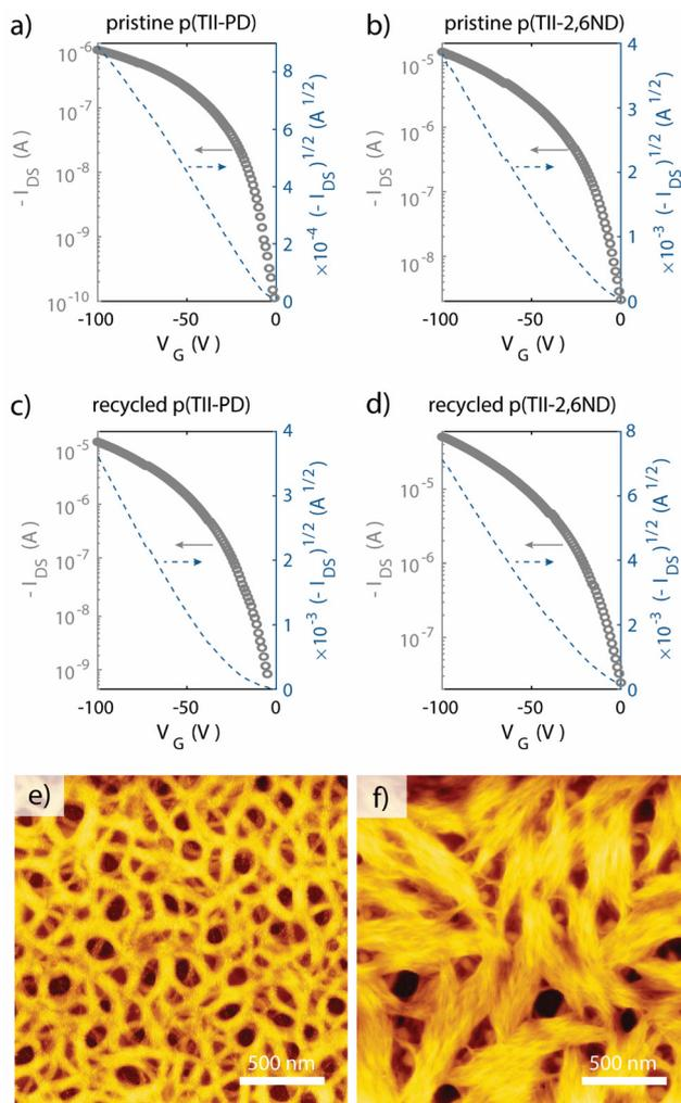
**Fig. 5** Typical transfer curves of pristine polymers (a) pristine p(TII-PD) and (b) pristine p(TII-2,6ND) and recycled polymers (c) re-p(TII-PD) and (d) re-p(TII-2,6ND). AFM height images of thin films of (e) p(TII-PD) and (f) p(TII-2,6ND) with 500 nm scale bar.
