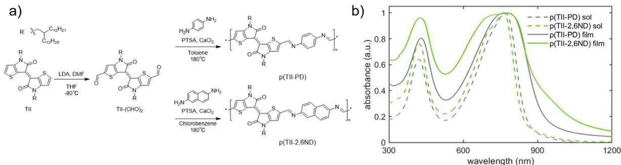
**Fig. 2** (a) Synthetic scheme of TII-(CHO)<sub>2</sub> and TII polymers; (b) UV-vis-NIR spectra of polymer solutions (in chlorobenzene) and thin films.
