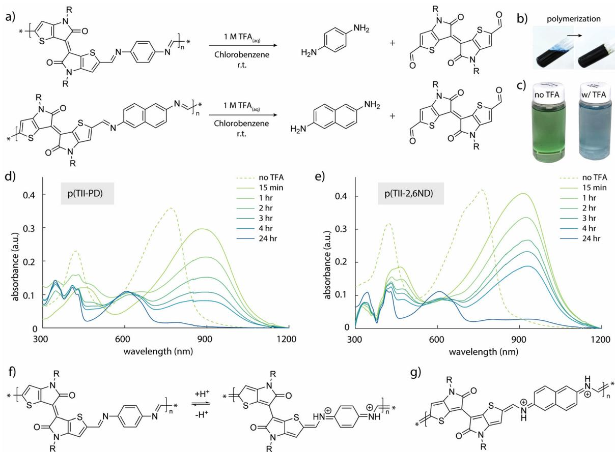
**Fig. 3** Degradation studies: (a) synthetic scheme of polymer degradation; (b) pictures taken before and after polymerization of p(TII-PD); (c) pictures taken before and after depolymerization of p(TII-PD) with TFA solution; UV-vis-NIR spectra during polymer degradation of (d) p(TII-PD) and (e) p(TII-2,6ND); the protonated aromatic-quinoidal transition for (f) p(TII-PD) and (g) p(TII-2,6ND), leading to red-shifted UV-vis-NIR spectra.
