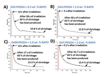
Fig. 3 Rheometer-monitored graphs of the bio-based acrylate copolymers over time under LED light (405 nm): (A) DAS: PEGDA with 0.5 wt% of BAPO (photoinitiator); (B) DAS: PEGDA with 2 wt% of BAPO; (C) DAM: PEGDA with 2 wt% of BAPO; and (D) DAT: PEGDA with 2 wt% of BAPO. The red line indicates the time when the lamp was turned on.
