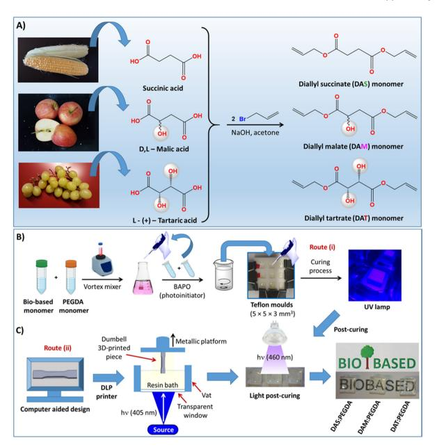
Fig. 1 (A) Illustration of the synthetic route followed to prepare the bio-based monomers: DAS, DAM and DAT. (B) Schematic representation of the procedure carried out for the copolymerization of the bio-based monomers and PEGDA co-monomer and the subsequent deposition inside Teflon moulds and curing under light. (C) Representation of the scale-up production of dumbbell test specimens in a DLP printer and the post-curing process in controlled visible light.
