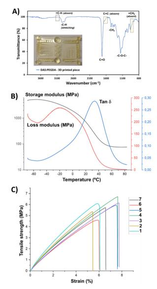
Fig. 7 (A) FTIR-ATR spectrum of the 3D-printed piece shown in the inset image. (B) DMA analysis of the DAS: PEGDA copolymer. (C) Stressstrain curves of DAS: PEGDA copolymer dumbbell samples. Both assays were performed with samples DLP printed under UV light and after post-curing processes.
