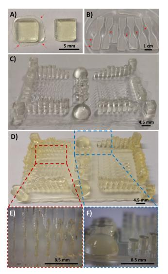
Fig. 6 Examples of some pieces printed with the DLP 3D printer employing the bio-based resin DAS and PEGDA monomer: (A) square bar samples used for biodegradability assays. (B) Dumbbell-shaped probes for stressstrain experiments. (C) Details of the dimensional stability of the resolution piece. Arrows in (A and B) indicate the bottom membrane that can be easily removed. (D) Resolution piece after the post-curing processes. (E and F) Details from the pillars and shapes printed.
