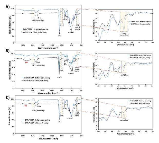
Fig. 4 FTIR-ATR spectra comparing the samples before and after the post-curing process: (A) DAS: PEGDA; (B) DAM: PEGDA; and (C) DAT: PEGDA copolymers. On the right, the detail of the =CH<sub>2</sub> out-of-plane bending bands, which overlapped evidencing that the polymerization reaction was complete.
