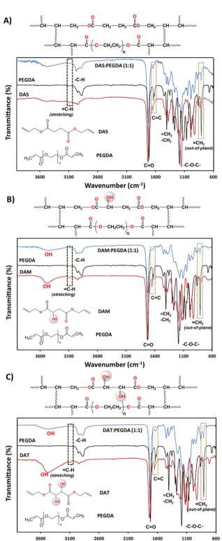
Fig. 2 Sequence of FTIR-ATR spectra comparing the monomers and the copolymer main functional groups: (A) DAS, PEGDA, DAS: PEGDA (1:1); (B) DAM, PEGDA, DAM: PEGDA (1:1); and (C) DAT, PEGDA, DAT: PEGDA (1:1). The reduction of double bond end groups, after UV photopolymerization, and the chemical structures of the copolymers are highlighted.
