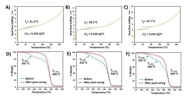
Fig. 5 DSC analysis showing the second heating curves used to determine the glass-transition temperatures and heat capacities of: (A) the DAS: PEGDA sample; (B) the DAM: PEGDA sample; and (C) the DAT: PEGDA sample. TGA curves, illustrating the main degradation steps, before and after complete curing, for: (D) the DAS: PEGDA sample; (E) the DAM: PEGDA sample; and (F) the DAT: PEGDA sample.
