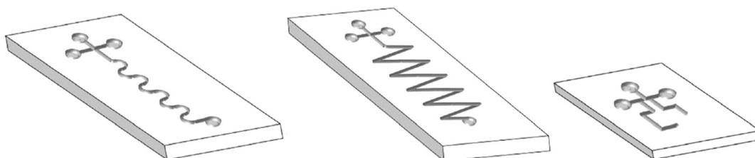
Fig. 16 Micromixer designs used for wastewater treatment.
