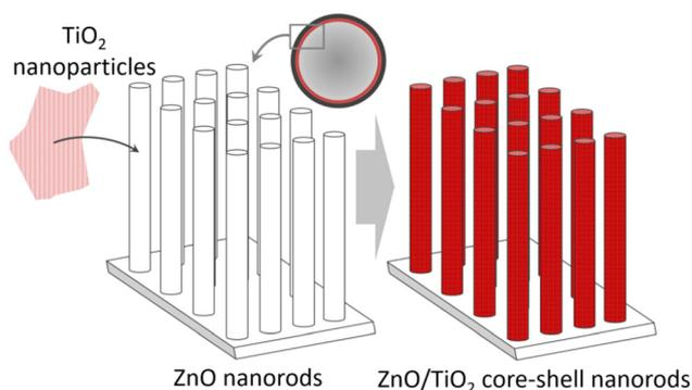
Fig. 8 TiO<sub>2</sub> nanoparticle-coated ZnO nanorod arrays grown in the capillaries of a photocatalytic microreactor.
