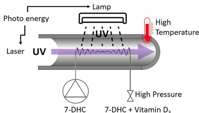
Fig. 18 Scheme of continuous flow photo-high- $p,T$  intensification reactor.<sup>83</sup>
