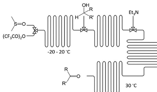
Fig. 3 Flow chemistry applied to sequential multi-step Swern-Moffatt-type oxidation.
