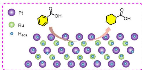
Fig. 21 Schematic diagram for the electroreduction of benzoic acid to cyclohexanecarboxylic acid over the Pt<sub>1</sub>Ru<sub>1.5</sub> catalyst.
