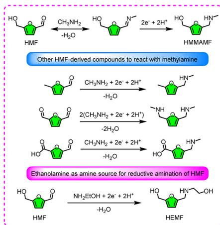
Fig. 8 The electrocatalytic reductive amination of 5-hydroxymethylfurfural (HMF).
