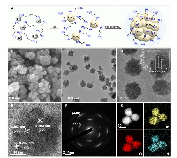
Fig. 1 Synthesis and morphology of amine-functionalized In<sub>2</sub>O<sub>3</sub> nanocrystals. (A) Schematic of the synthetic route. (B) SEM images. (C)–(E) TEM images, particle size distribution (inset) and HRTEM images. (F) SAED pattern. (G) EDS mapping
