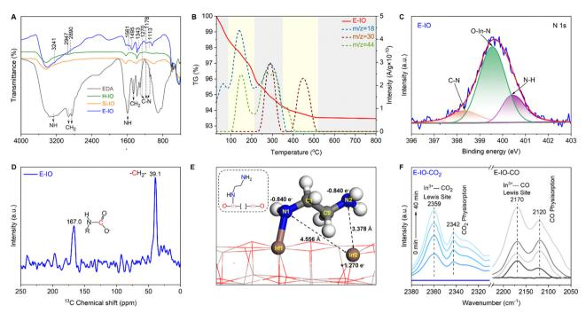
Fig. 2 Characterization of samples (A) FTIR spectra of H-IO, Si-IO and E-IO. (B) TGA-MS curves of E-IO in air condition. (C) High resolution N 1s XPS spectra of E-IO. (D) 13C MAS NMR spectra of E-IO at room temperature. (E) Optimized structure of the grafting state InNH2···In. (F) In situ DRIFTS spectra of the adsorption of CO2 (left) and CO (right) on the E-IO surface at 298 K.
