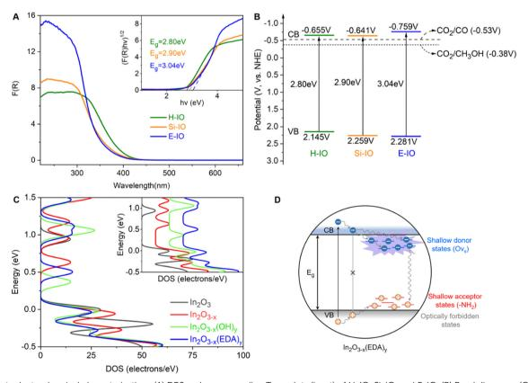
Fig. 4 Photoelectrochemical characterizations (A) DRS and corresponding Tauc plots (inset) of H-IO, Si-IO, and E-IO. (B) Band diagrams. (C) The total DOS for  $ln_2O_3$ ,  $ln_2O_{3-x}$ ,  $ln_2O_{3-x}$  (DH)<sub>v</sub>, and  $ln_2O_{3-x}$  (EDA)<sub>v</sub> (110) surface, expanded view of the DOS in the conduction band region (inset). (D) A schematic illustration of charge carrier recombination pathways in  $In_2O_{3-x}(EDA)_y$  nanoparticles.
