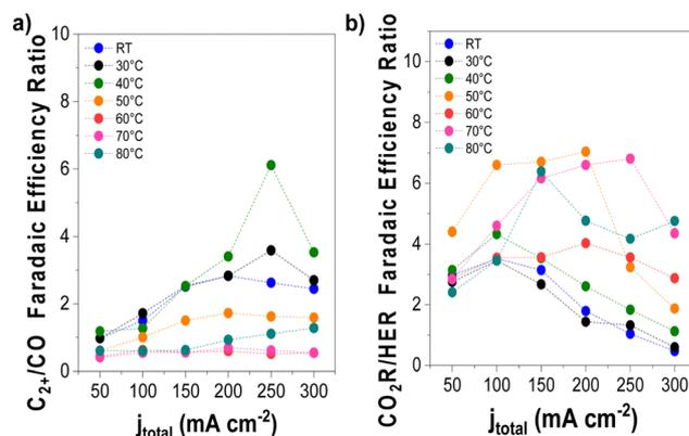
Fig. 4 Selectivity trends as a function of operating temperature and applied current density. (a) C<sub>2+</sub>/CO and (b) CO<sub>2</sub>-derived products/H<sub>2</sub> FE ratio. Experimental conditions: Cu-GDE (cathode), MPIP-AEM, IrO<sub>2</sub> (anode), CO<sub>2</sub> feeding rate 20 sccm, 0.1 M KHCO<sub>3</sub> as anolyte. Results are paired with those presented in Fig. 5.
