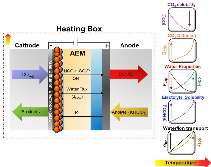
Fig. 1 Schematic representation of temperature dependency on transport and kinetics properties on  $CO_2E$  in zero-gap configuration. Equations for the presented trends for the different properties can be found in the ESI.<sup>†</sup>
