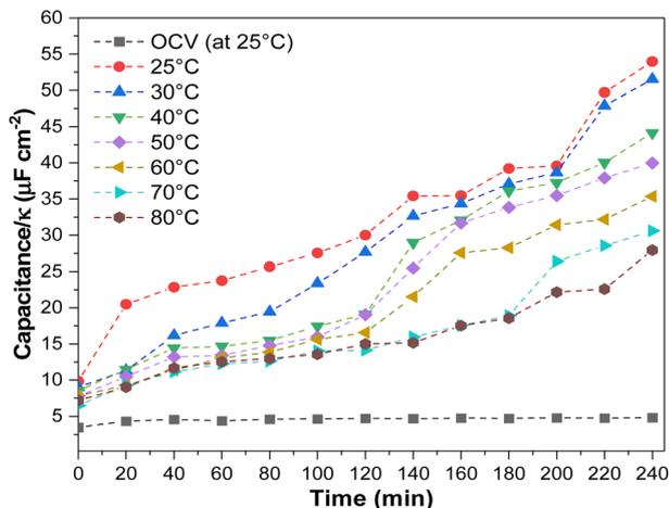
Fig. 7 Tracking the electrode flooding by DLC measurements as a function of the operating temperature at  $200 \text{ mA cm}^{-2}$ . OCV was conducted at room temperature. Experimental conditions: Cu-GDE (Cathode), MPIP-AEM,  $\text{IrO}_2$  (Anode),  $\text{CO}_2$  flow rate: 20 sccm, 0.1 M  $\text{KHCO}_3$  as anolyte.
