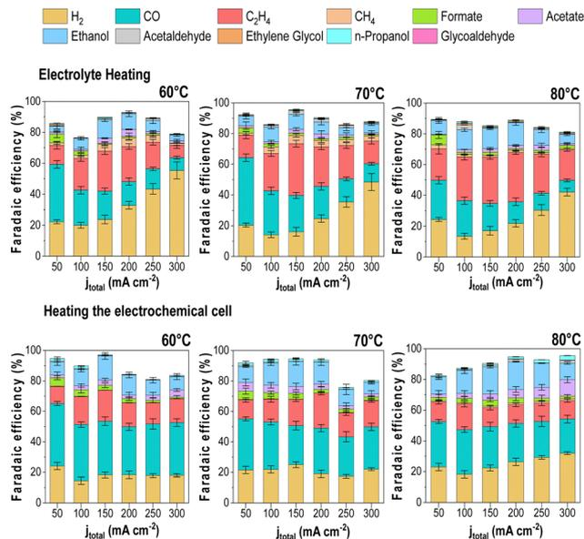
Fig. 8 Effect of the cell heating in the product distribution using two different methods at different operating temperatures experimental conditions: Cu-GDE (Cathode), MPIP-AEM,  $\text{IrO}_2$  (Anode),  $\text{CO}_2$  flow rate: 20 sccm, 0.1 M  $\text{KHCO}_3$  as anolyte. Error bars represent the standard error of the independent measurements at each different condition.
