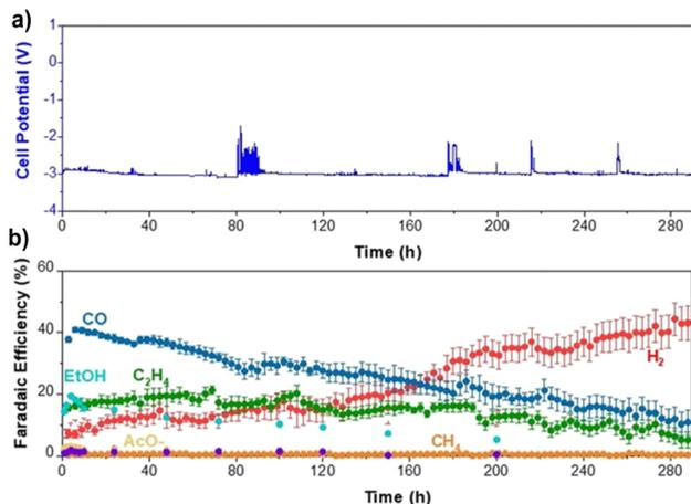
**Fig. 10** 290 hour CO<sub>2</sub> electrolysis stability test at 60 °C and 200 mA cm<sup>-2</sup>. (a) Potential profile. (b) Faradaic efficiency. Operating parameters were sputtered Cu cathode with 10% by weight MPIP ionomer, MPIP membrane, IrO<sub>2</sub> on carbon anode and 0.1 M CsHCO<sub>3</sub> as an electrolyte. 100 mbar back pressure on the cathode was used as well. Error bars represent the standard error of different injections and measured samples.
