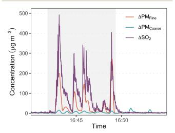
**Fig. 3** Time series tracking a high emission vehicle in Outer London. The grey shaded area represents the time period during which the vehicle was being measured.
