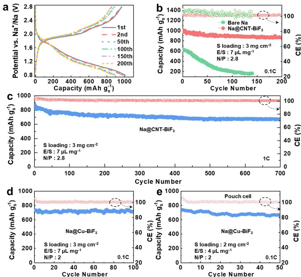
Fig. 7 Electrochemical performance of Na@CNT-BiF<sub>3</sub> and Na@Cu-BiF<sub>3</sub>. (a) Voltage profiles of Na@CNT-BiF<sub>3</sub> at various cycles. (b) Cycling performances of bare Na and Na@CNT-BiF<sub>3</sub> electrodes at 0.1C rate. (c) Cycling performance of Na@CNT-BiF<sub>3</sub> electrodes at 1C rate. Cycling performances of Na@Cu-BiF<sub>3</sub> electrodes in (d) coin cell and (e) pouch cell at 0.1C rate.
