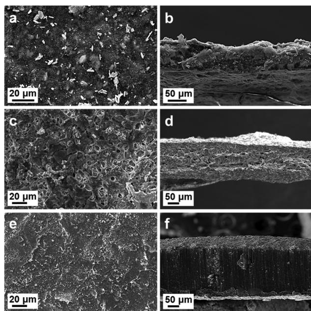
Fig. 3 Morphological characterization of the anode. Top-surface SEM of (a) BiF<sub>3</sub>-CNT, (c) Na@CNT-BiF<sub>3</sub> after cycling, and (e) Na@CNT-BiF<sub>3</sub> (after 200 cycles). Cross-sectional morphologies of (b) BiF<sub>3</sub> before cycling, (d) Na@CNT-BiF<sub>3</sub> (before cycling), and (f) Na@CNT-BiF<sub>3</sub> (after 200 cycles).
