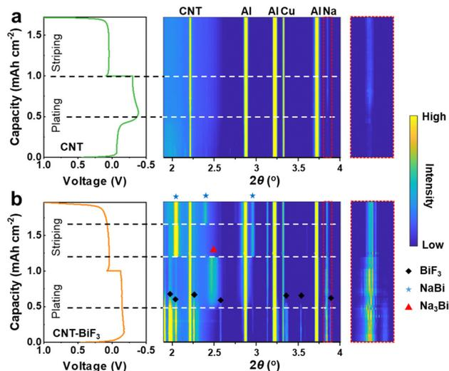
Fig. 5 *In operando* X-ray diffraction (XRD) characterization. Charge and discharge curves of (a) Na@CNT||Na@CNT and (b) Na@CNT-BiF<sub>3</sub>||Na@CNT-BiF<sub>3</sub> coin cell and the corresponding diffraction patterns.
