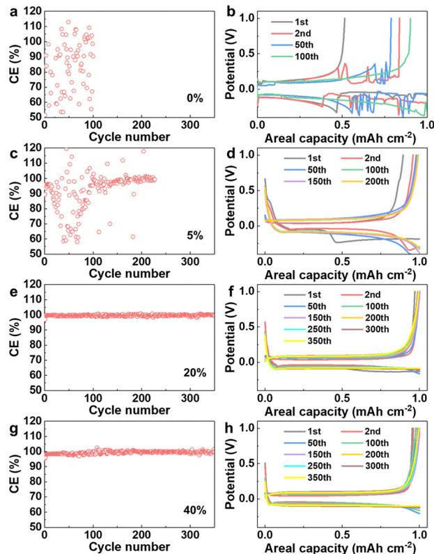
Fig. 6 Characterization and electrochemical performance of Cu- $\text{BiF}_3$  anodes. Coulombic efficiency and voltage-capacity curves of Na plating/stripping in (a) and (b) Cu-0%  $\text{BiF}_3$ , (c) and (d) Cu-5%  $\text{BiF}_3$ , (e) and (f) Cu-20%  $\text{BiF}_3$  (g) and (h) Cu-40%  $\text{BiF}_3$  at  $1 \text{ mA cm}^{-2}$ .
