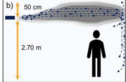
Fig. 1 Comparison of dosing  $O_3$  gas,  $H_2O_2$ , or TEG aerosols into the office room at (a) a medium height of about 1.5 m (without the Coandă effect), and (b) at 50 cm from the ceiling (at a height of 2.5 meters) with the Coandă effect.
