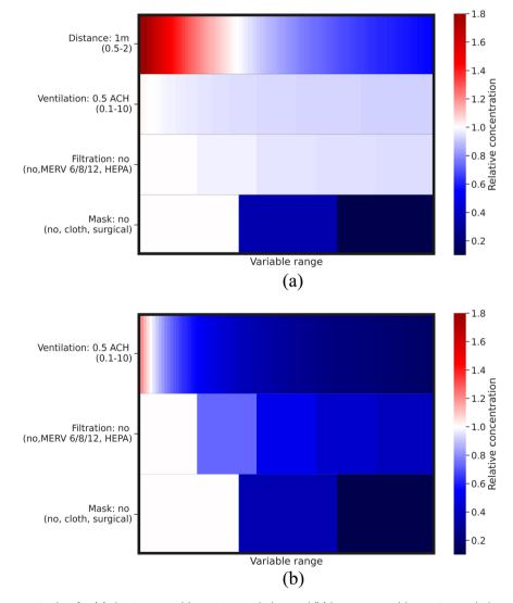
Fig. 6 Relative virus concentration for (a) short-range airborne transmission and (b) long-range airborne transmission, with the variable range referred to in Table 2.
