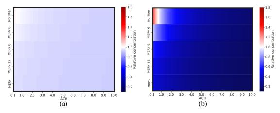
Fig. 7 Relative virus concentration compared to the base case as a function of different variable pairs for (a) short-range airborne transmission and (b) long-range airborne transmission.
