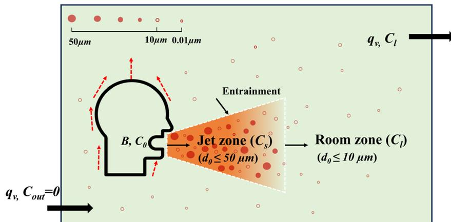
Fig. 1 A simple size-dependent model of the continuum from short-range to long-range inhalation routes (modified from Li *et al.*<sup>1</sup>).
