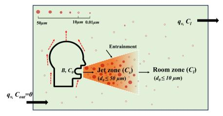
Fig. 1 A simple size-dependent model of the continuum from short-range to long-range inhalation routes (modified from Li et al.<sup>1</sup>).
