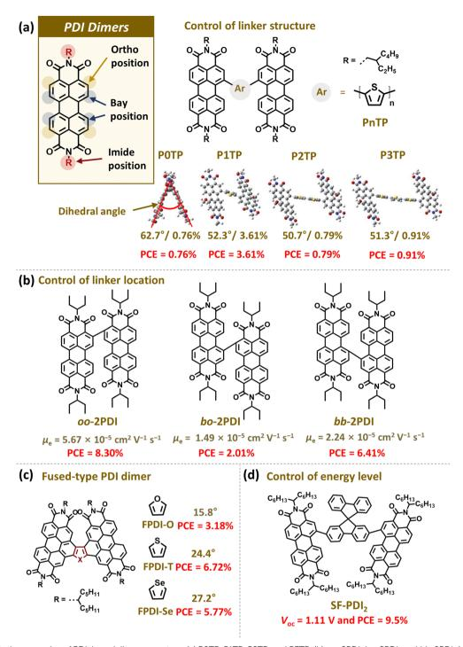
Fig. 5 Representative examples of PDI-based dimer acceptors; (a) POTP, P1TP, P2TP, and P3TP, (b) oo-2PDI, bo-2PDI, and bb-2PDI, (c) FPDI-O, FPDI-T, and FDPI-Se, and (d) SF-PDI<sub>2</sub>. Reproduced from ref. 121 with permission from the Royal Society of Chemistry, copyright 2024.
