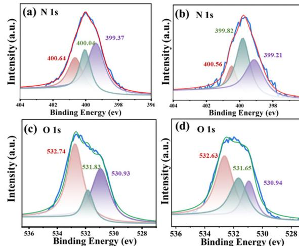
**Fig. 3** High-resolution N 1s XPS spectrum of (a) DvDf-C3XJ-COF and (b) DvDf-C3XJ-COF + Hg<sup>2+</sup>. High-resolution O 1s XPS spectrum of (c) DvDf-C3XJ-COF and (d) DvDf-C3XJ-COF + Hg<sup>2+</sup>.
