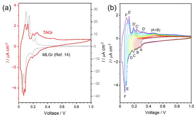
**Fig. 3** (a) The 3rd CV curves of SE-cells using a TAGr (red, left y-axis) and an MLGr (gray, right y-axis (after ref. 14)) at 25 °C. (b) CV curves for a SE-cell using a TAGr. The voltage was swept from 1.00 V to the desired values (0.02, 0.06, 0.08, 0.10, 0.12, 0.14, 0.16, 0.18, 0.20, 0.22, 0.24, 0.26, 0.28, 0.30 V) and then swept to 1.00 V, respectively.  $v = 0.5 \text{ mV s}^{-1}$ .
