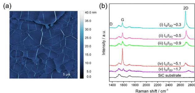
Fig. 2 (a) Topographic AFM image of TAGr grown on a SiC(000 $\bar{1}$ ) substrate. (b) Raman spectra of the TAGr and SiC(000 $\bar{1}$ ) substrate. Each spectrum was measured at different points in the same sample.
