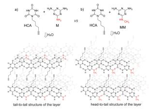
Fig. 1 Layered structures formed by self-assembly of hexynil cyanuric acid with (a) melamine and (b) N-methylmelamine.
