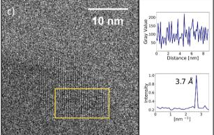
Fig. 3 (a) TEM images of M\*HCA. The profiles were taken along long axes and averaging was performed along the short axes of the yellow rectangles. The inserts show the resulting profiles, their FFT, and the characteristic periodicity. (b) and (c) Cryo-TEM images of MM\*HCA. The analysis was performed similarly to (a).
