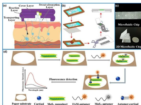
**Fig. 8** Schematic representation of the fabricated 3D origami microfluidic device (a) sweat channels, (b) 3D microfluidic origami chip, (c) four-layered microfluidic origami chip, (d)  $\text{MoS}_2$ -mediated FRET device. Reproduced from ref. 81 with permission from American Chemical Society, copyright 2022.
