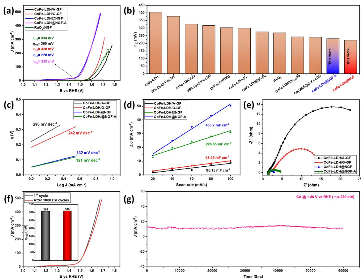
Fig. 4  $iR$ -corrected polarization curves (a), comparison of CoFe-LDH@NGF with literature reports (b), comparison of Tafel plots (c), double layer capacitance ( $C_{dl}$ ) at different scan rates (d), and EIS Nyquist spectra (e) of CoFe-LDH@A-GF, CoFe-LDH@O-GF, CoFe-LDH@NGF and CoFe-LDH@NGF-A in 1.0 M KOH. Comparison of LSV curves (f) and  $\eta_{100}$  (inset) before and after 1000 CV cycles (g). Chronoamperometry analysis performed at overpotential of 230 mV.
