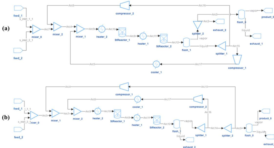
Fig. 11 Optimal flowsheets for HDA system with 20 units in pool. (a) product purity = 99.9%, product flow rate =  $0.240 \text{ mol s}^{-1}$ ; (b) product purity = 95.9%, product flow rate =  $0.288 \text{ mol s}^{-1}$ .
