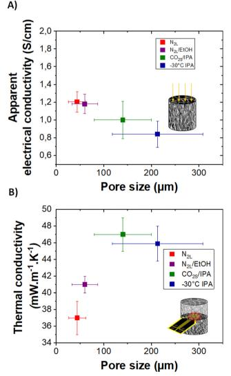
Fig. 7 (A) and (B) Apparent electrical conductivity and thermal conductivity of templated cryogels with different pore sizes, respectively
