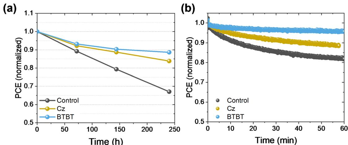
Fig. 5 Stability test on PSCs without encapsulation in (a) ambient conditions (25% RH) and (b) under continuous illumination and MPPT conditions.
