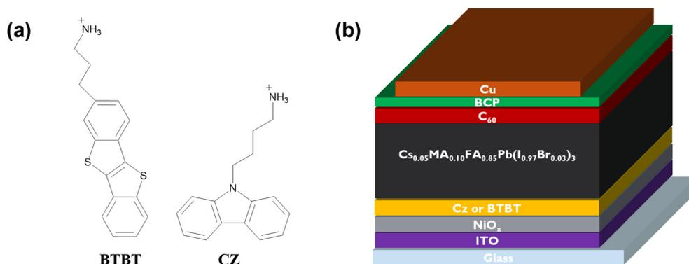
Fig. 1 (a) Molecular structure of BTBT and Cz. (b) Perovskite solar cell stack depiction. The control sample does not contain any modification between NiO<sub>x</sub> and the perovskite layer.
