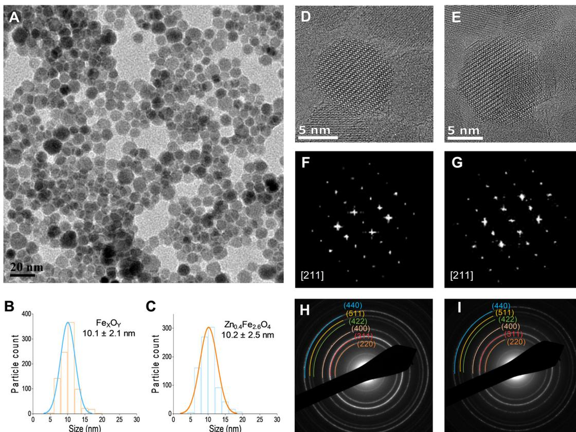
Fig. 1 (A) TEM image of  $\text{Zn}_{0.4}\text{Fe}_{2.6}\text{O}_4$  NPs prepared under high temperature with autogenous pressure; (B) and (C) size distributions; (D) and (E) HRTEM images; (F) and (G) FFT patterns down the [211] axis; and (H) and (I) selected area electron diffraction (SAED) patterns with denoted crystal planes for iron oxide and  $\text{Zn}_{0.4}\text{Fe}_{2.6}\text{O}_4$  NPs respectively.
