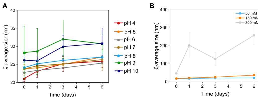
Fig. 4 Colloidal stability of  $\text{Zn}_{0.4}\text{Fe}_{2.6}\text{O}_4$  NPs at (A) different pH values and (B) a range of electrolyte concentrations ( $n = 3$ ).
