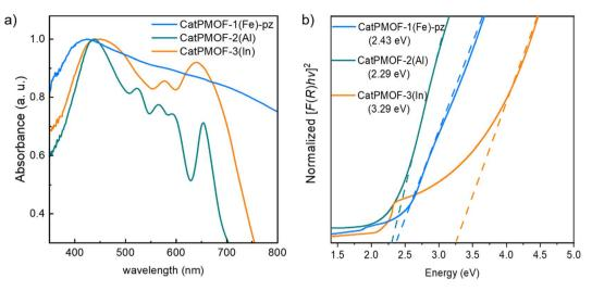
Fig. 6 Solid-state UV-visible absorption spectra (a) and normalized Tauc plot of the Kubelka–Munk-transformed data (b) for CatPMOF-1(Fe)-pz, CatPMOF-2(Al) and CatPMOF-3(In). Dashed lines indicate linear fits to the absorption onsets (b).
