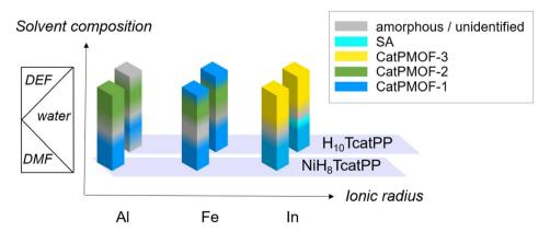
Fig. 1 Qualitative phase diagram in the systems NiH $_8$ TcatPP-M(III) and H $_{10}$ TcatPP-M(IIII): influence of the nature of the cation and the solvent mixture (for synthesis at 150-160 °C).
