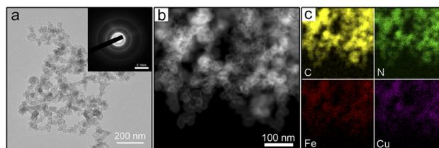
Fig. 1 (a) TEM and SAED (inset) images of FeCu-SAC. (b) HAADF-STEM image of FeCu-SAC. (c) EDX elemental maps of FeCu-SAC.
