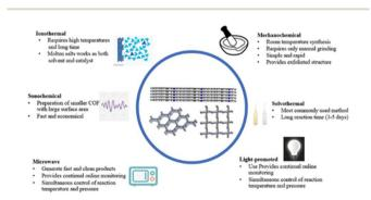
Fig. 2 Common synthesis methods of COFs.
