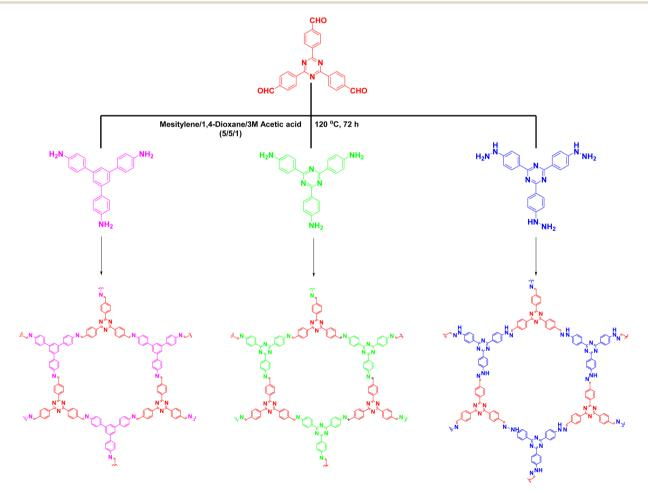
Fig. 10 COFs were synthesized by reaction of different nitrogenous building blocks with 4,4',4"-(1,3,5-triazine-2,4,6-triyl) Schiff bases.
