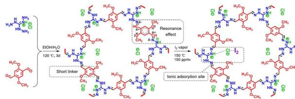
Fig. 6 Schematic of the design and synthesis of ionic COF TGDM and explanation of its high stability and I<sub>2</sub> uptake mechanism. Reproduced with permission from ref. 84. Copyright 2022, American Chemical Society. The ionic sites (quaternary ammonium) strongly interact with [I<sub>2</sub>Cl]<sup>-</sup> species through Coulomb forces.
