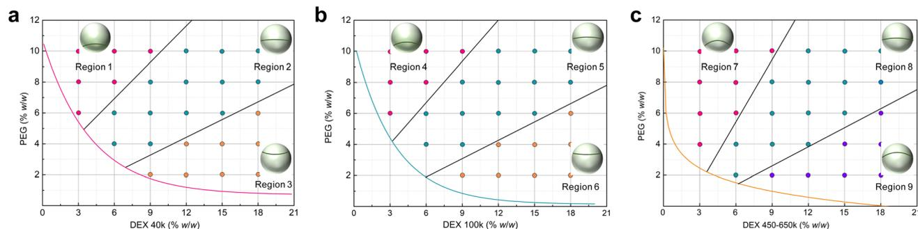
**Fig. 3** Dividing each phase diagram into three representative regions above the binodal curve to represent the resultant ATPS Janus droplets using accordingly simulated morphologies (inset pictures). These phase diagrams represent the Janus droplet formed by PEG 20k and DEX 40k aqueous solutions (a), PEG 20k and DEX 100k aqueous solutions (b), PEG 20k and DEX 450–650k aqueous solutions (c), respectively.
