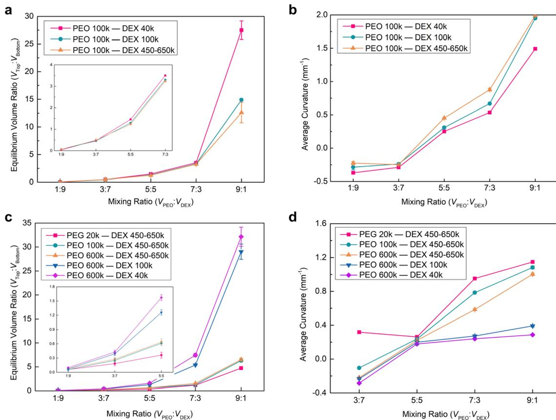
Fig. 4 The volume ratio of the top and bottom phases and interfacial curvature in the Janus droplets versus the mixing ratio of 10% w/w PEO 100k and 15% w/w DEX (40k, 100k and 450–650k) (a and b), 5% w/w PEO (20k, 100k and 600k) and 15% w/w DEX 450–650k (c and d) aqueous solutions.
