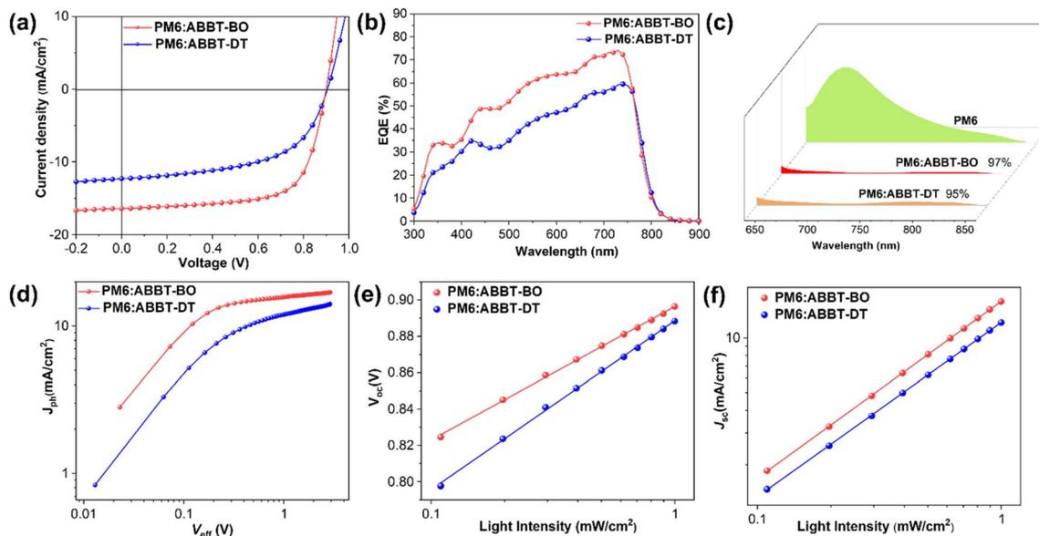
Fig. 3 (a)  $J$ - $V$  characteristics and (b) EQE spectra of the optimal OSCs. (c) PL spectra of PM6 and PM6:NFA blend films. (d)  $J_{\text{ph}}$ - $V_{\text{eff}}$  relationships of PM6:ABBT-BO and PM6:ABBT-DT. (e)  $V_{\text{OC}}$  versus light intensity curves and (f)  $J_{\text{SC}}$  versus light intensity curves of PM6:ABBT-BO and PM6:ABBT-DT.
