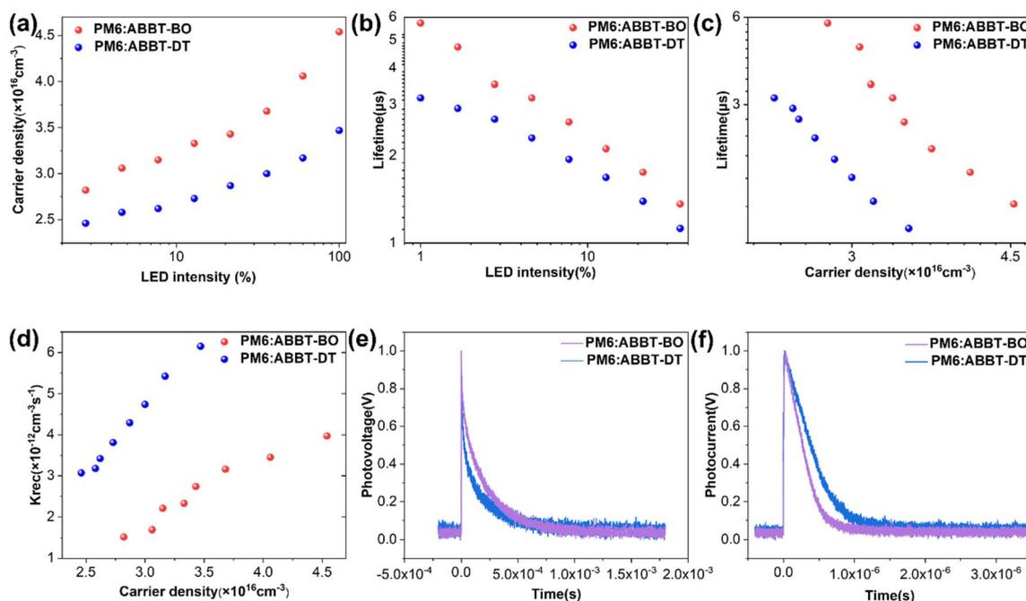
Fig. 4 (a) Charge density versus light intensity. (b) The carrier lifetimes and densities under different illumination intensities. (c) Charge lifetime versus charge density. (d) Bimolecular recombination rate constant  $k_{rec}$  extracted from  $\tau$  and  $n$ . (e) TPV and (f) TPC characterization of **PM6:ABBT-BO** and **PM6:ABBT-DT**.
