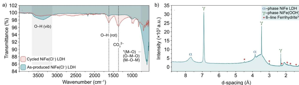
Fig. 6 (a) FT-IR spectra of pre-cycled (black line) and post-cycled (red line)  $\text{Cl}^-$ -intercalated NiFe LDH and (b) XRD pattern for NiFe LDH after 200 cycles between  $1.02\text{--}1.62\text{ V}$  vs. RHE at  $5\text{ mV s}^{-1}$ . The  $\alpha$ -NiFe LDH and  $\gamma$ -NiFeOOH phases are labelled, as well as a ferrihydrite signal at low  $d$ -spacing.<sup>1</sup>
