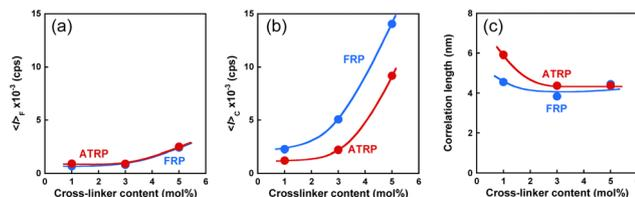
Fig. 4 The effect of the cross-linker content on (a)  $\langle I \rangle_F$ , (b)  $\langle I \rangle_C$ , and (c)  $\xi$  of the ATRP and FRP gels at 25 °C. Their gels were synthesized with various cross-linker content at 5 °C.
