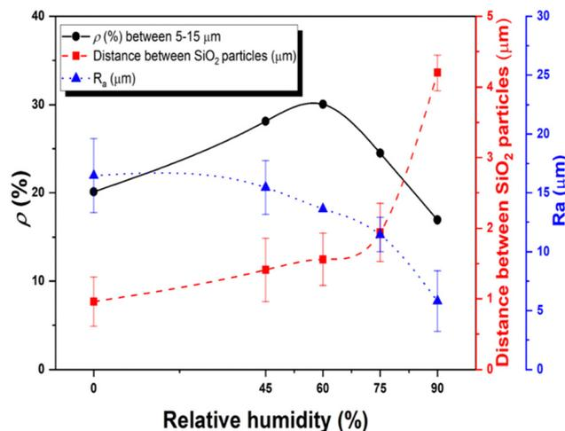
Fig. 3 Relationship between the percentage of infrared radiation emitted by the human body that is reflected by the PNIPAM-based hydrogel composite containing 20 wt% of  $\text{SiO}_2$  (black circles), the distance between the  $\text{SiO}_2$  particles (red squares) and the surface roughness (blue triangles) with respect to the relative humidity.
