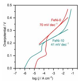
Fig. 5 Tafel plots of pristine nickel hydroxide (FeNi-0) and ironincorporated nickel hydroxide (FeNi-10) electrocatalysts measured in an alkaline medium (1.0 M NaOH) at 1.0 mV  $s^{-1}$  scan rate
