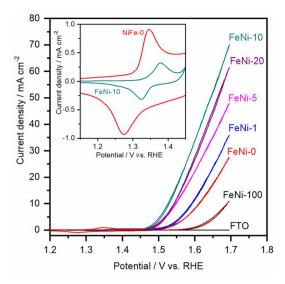
Fig. 3 LSV curves for pristine nickel hydroxide (FeNi-0), iron hydroxide (FeNi-100), and iron-incorporated nickel hydroxide electrodes measured in an alkaline medium (1.0 M NaOH) without iR-compensation and at a scan rate of 5 mV  $s^{-1}$
