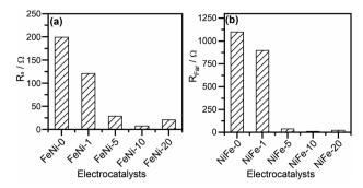
Fig. 7 (a) Intermediates' formation resistance  $(R_s)$  and (b) the faradaic resistance ( $R_{Far} = R_s + R_p$ ) for pristine and iron-incorporated nickel hydroxide electrodes calculated by fitting the Nyquist plots presented in Fig. 6a with the EC in Fig. 6b.
