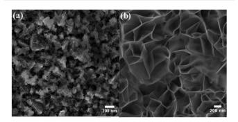
Fig. 1 SEM images of (a) iron-incorporated nickel hydroxide (FeNi-10) and (b) pristine nickel hydroxide (FeNi-0) films.
