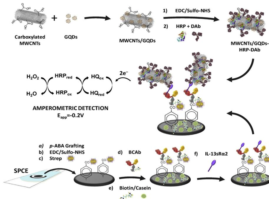
Fig. 7 Scheme for the detection of IL-13sR $\alpha$ 2 by a sandwich amperometric immunosensor using MWCNT/GQD-HRP-DAB nanocarriers. Reproduced from ref. 142 with permission from Elsevier, copyright [2017].<sup>142</sup>
