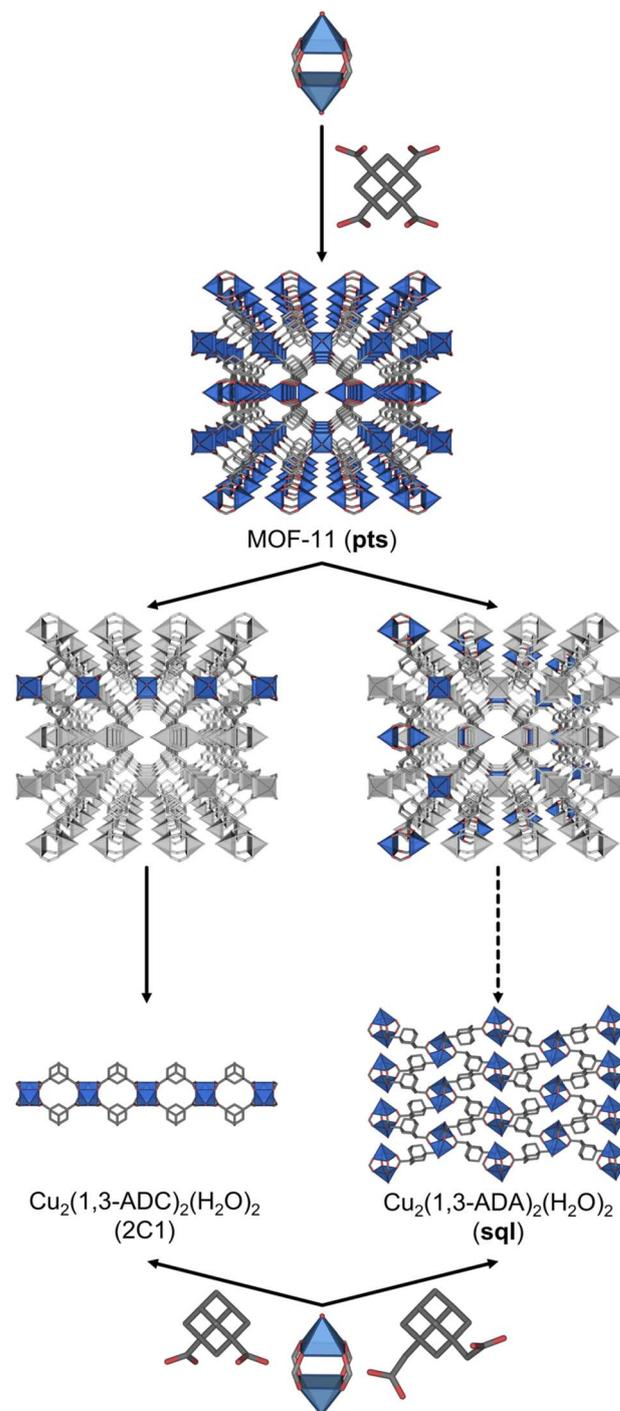
Fig. 2 Schematic of the net-clipping approach applied to the formation of metal–organic materials from tetrahedral 1,3,5,7-ATC linker to turned-twisted 1,3-ADC (left) or 1,3-ADA (right) linkers combined with 4-c paddlewheel Cu(II) MBBs.
