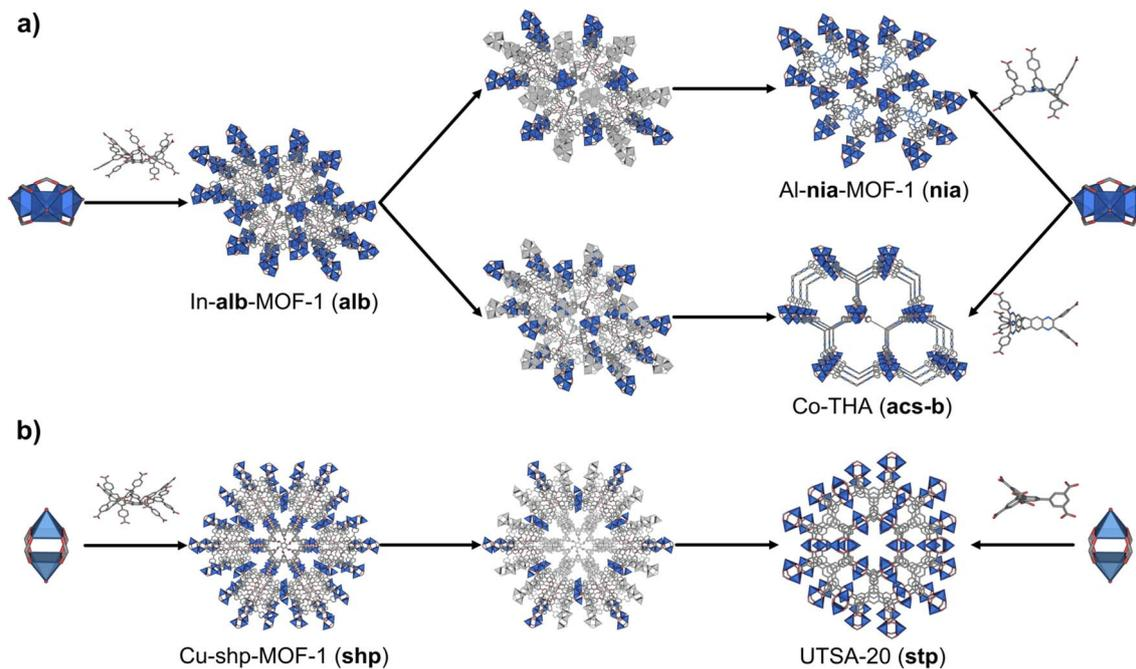
Fig. 5 Schematic of the net-clipping approach applied to formation of metal–organic materials from (a) a hexagonal prism BCPB linker clipped to an octahedral TTATTDC, and trigonal prism THA linkers combined with a 6-c trimer  $M_{(III)}$  MBBs; and (b) a hexagonal prism BCPB linker clipped to a distorted trigonal prism BHB linker, combined with 4-c paddlewheel  $Cu_{(II)}$  MBBs.
