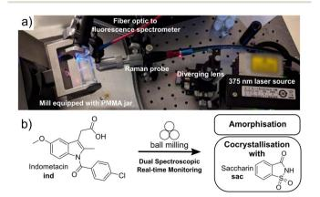
Fig. 1 (a) Instrumental setup for tandem time-resolved *in situ* monitoring of milling reactions using solid-state fluorescence emission and Raman spectroscopies. (b) Model mechanochemical transformations monitored in this work: amorphisation and cocrystallisation of indometacin (ind).
