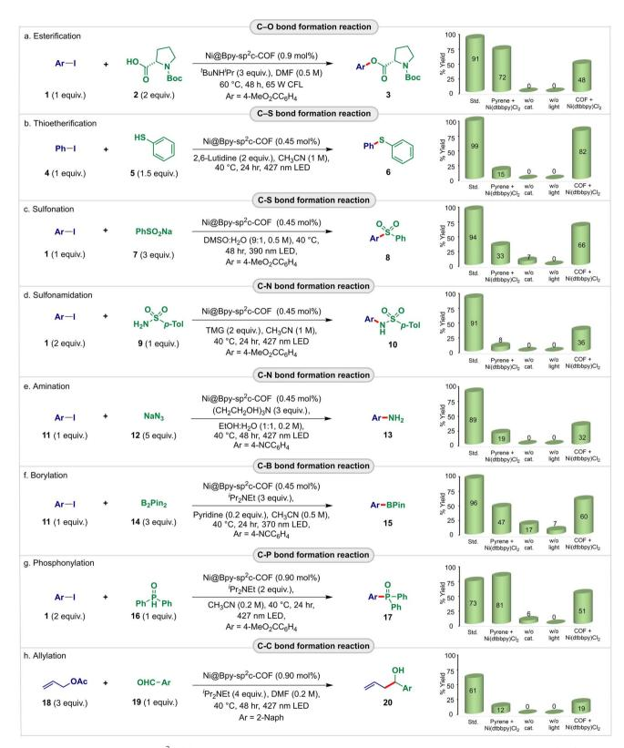
Fig. 3 Exploration of the Ni@Bpy-sp $^2$ c-COF as the dual interlocked catalyst for the light-harvesting cross-coupling reactions (a–h). Reactions were performed at 0.1 mmol scales. Std conditions as defined in the equation. Homogeneous controls were performed with pyrene/(dtbbpy) NiCl $_2$  (5 mol $_2$ ). Semi-heterogeneous controls were performed with Bpy-sp $^2$ c-COF/(dtbbpy)NiCl $_2$  having the same loading as std conditions. See Tables S2–S17 $_1$  for details.
