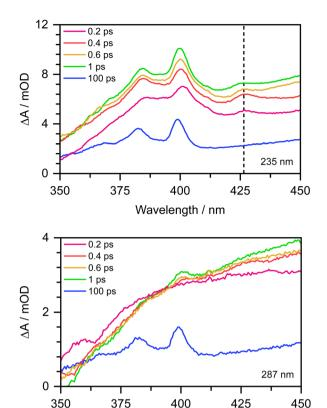
Fig. 7 350–450 nm transient absorption spectra of 20 mM aqueous phenolate at displayed pump-probe delays following photoexcitation at 235 nm (top) and 287 nm (bottom). The dashed vertical highlights the peak at 427 nm described in the main text.
