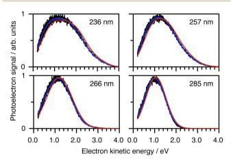
Fig. 4 Resonance-enhanced 1 + 1 photoelectron spectra (PES) of aqueous phenolate at 236, 257, 266 and 285 nm (black) together with retrieved true PES (solid red lines).<sup>31</sup> The 285 nm spectrum is adapted according to CC-BY license from ref. 31. Copyright 2022 the authors. Published by American Chemical Society under a Creative Commons CC BY 4.0 license.
