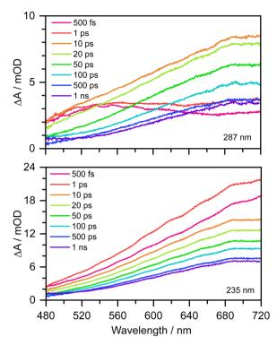
Fig. 2  $\,$  480–720 nm transient absorption spectra of 20 mM aqueous phenolate at displayed pump-probe delays following photoexcitation at 287 nm (top) and 235 nm (bottom). The broad absorption centered around 700 nm is attributed to solvated electrons and the absorption feature with a peak around 540 nm is attributed to the S $_1$  state of phenolate.  $^{12}$
