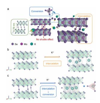
Fig. 1 (a) Schematic illustration of the modulation of Se–Se bonds. (b and c) Crystal structure and mechanism of MoSe<sub>2</sub> and MoSe<sub>2+x</sub>, respectively. Purple atoms represent selenium, pink atoms represent molybdenum, and green atoms represent potassium.
