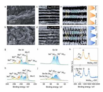
Fig. 2 Morphology and structure characterization. SEM images of (a)  $MoSe_2-rGO$  and (b)  $MoSe_{2+x}-rGO$ . HRTEM images of (c)  $MoSe_2-rGO$  and (d)  $MoSe_{2+x}-rGO$ . Atomic images of (e)  $MoSe_2-rGO$  and (f)  $MoSe_{2+x}-rGO$ ; the line scan profiles along the corresponding rectangles are shown on the right. XPS spectra of (g and i)  $MoSe_2-rGO$  and (h and j)  $MoSe_{2+x}-rGO$ . (k) Raman spectra of  $MoSe_2-rGO$  and  $MoSe_{2+x}-rGO$ .
