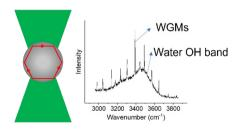
Whispering Gallery Modes (WGMs) can be used to determine droplet size and refractive index.
